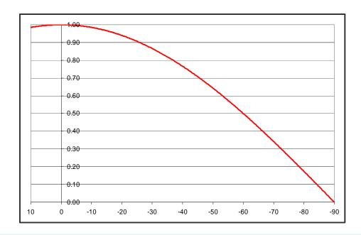
Here is the elevation pattern of a single FML series antenna bay. It has an elevation gain of -0.48, or -3.20 dB. When the antenna is mounted 98 feet from the ground, the signal level 98 feet from the tower will be at a depression angle of -45 degrees, At 3 miles from the tower the beam from this antenna will be at -0.36 degrees.
