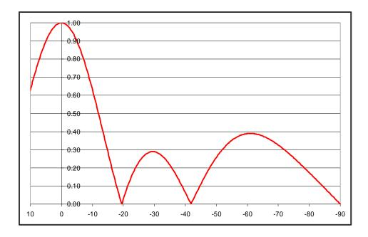
Here is the elevation pattern of a 3 bay FML series antenna. This antenna has an elevation gain of 1.52 (1.84 dB). When mounted 98 feet above the ground the first null is located at a depression angle of -19.50 degrees, which is 278 feet from the tower. The second null located at -42.00 degrees is located 109 feet from the tower.
