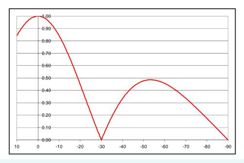
Here is the elevation pattern of a two bay **FML** series antenna. It has an elevation gain of 1.00 (0.00 dB). When mounted 98 feet above the ground the first null will fall 171 feet from the tower at a depression angle of -30 degrees.
