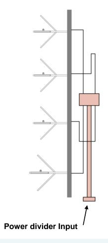
Pictured to the left is a depiction of a 4 bay branch fed FM antenna. Each bay is receiving 1/4<sup>th</sup> of the power that is presented to the input power divider. If each antenna bay has a rating of 4 kW, a properly sized input power divider would give a 16 kW input power rating for the array.
